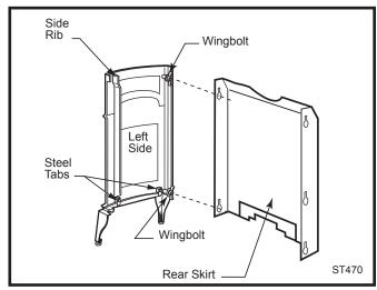
Fig. 3 Attach rear skirt to the left side.
